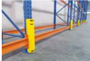
Protectors easily modified on site to fit around bottom beams
